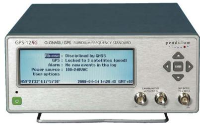
The Pendulum GPS-12RG Portable Reference clock is an ultra-stable GLONASS and GPS-disciplined Rubidium reference, targeted for both laboratory and telecommunications applications. The built-in battery option enables transportation of lab accuracy to field applications. When locked to GLONASS and/or GPS, its near-Cesium performance makes the GPS-12RG an ideal calibrator for metrology and test systems.
