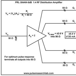
Fig. 1, PRL-304AN-0dB 1:4 RF Distribution Amplifier
